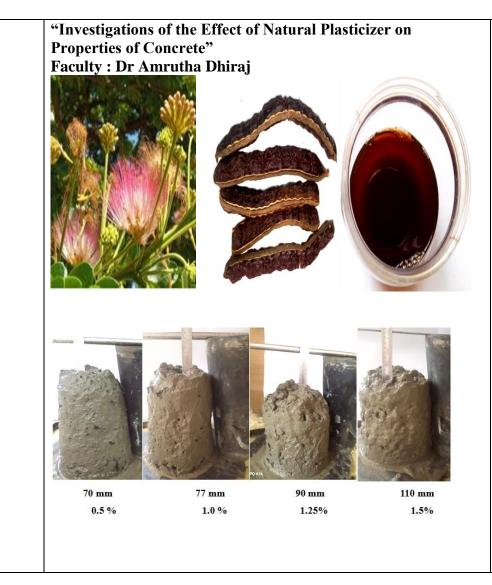
Admixtures are commonly used in construction to improve concrete properties. However, chemical plasticizers, which contain formaldehyde, pose environmental hazards.
