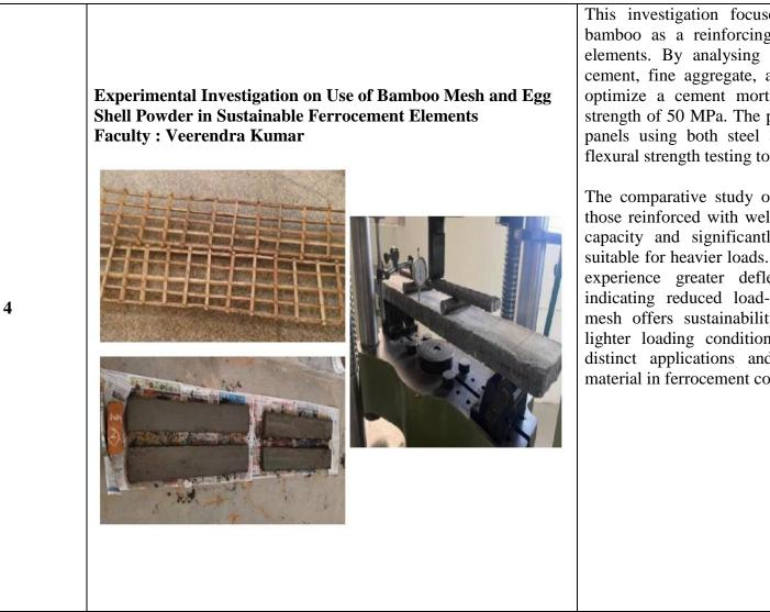
This investigation focuses on the experimental study of bamboo as a reinforcing mesh in sustainable ferrocement elements. By analysing the properties of key materials cement, fine aggregate, and bamboo—the research aims to optimize a cement mortar mix to achieve a compressive strength of 50 MPa. The project involves casting ferrocement panels using both steel and bamboo meshes, followed by flexural strength testing to compare their performance.
