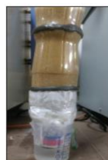
c) Sand and gravel layer and cloth layer compartment
