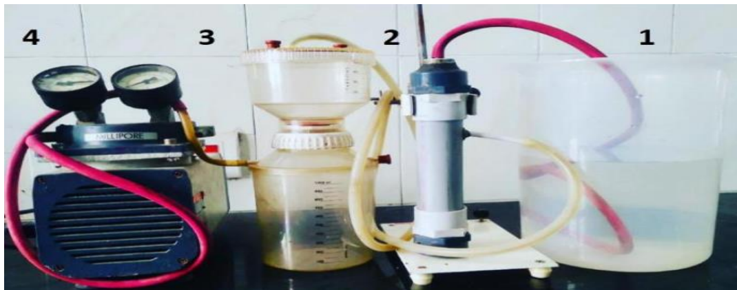
Fig 2.6 Experimental setup of portable water purifier
