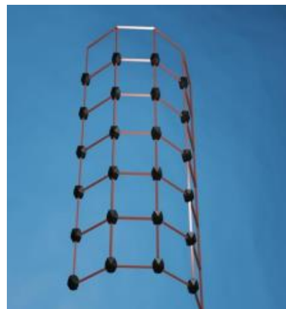
Fig 2.2 Coconut carbon fiber embedded on copper mesh
