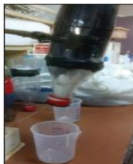
b) Activated charcoal layer and cotton layer compartment
