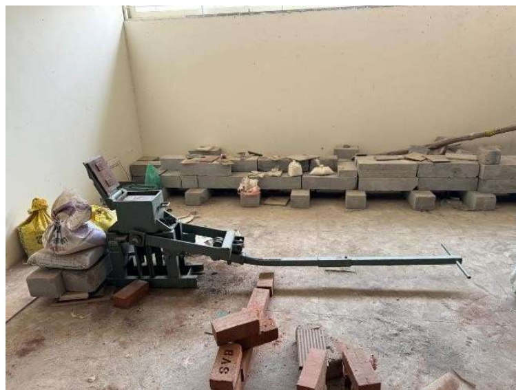
Fig 2.3: Mardini stabilized mud block press (KSSEM Laboratory)
