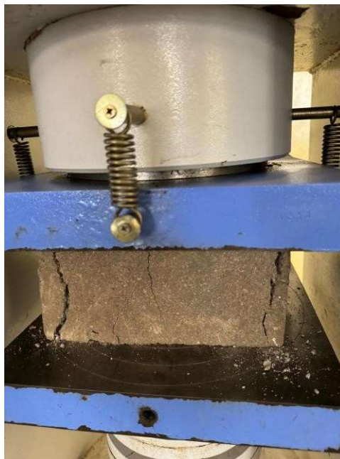
Figure 4. 1 Test Specimen of Block After Failure (KSSEM Laboratory)
