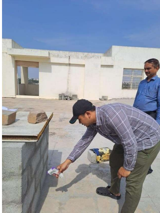
Figure 3.6 Recording Surface Temperature (KSSEM Laboratory)
