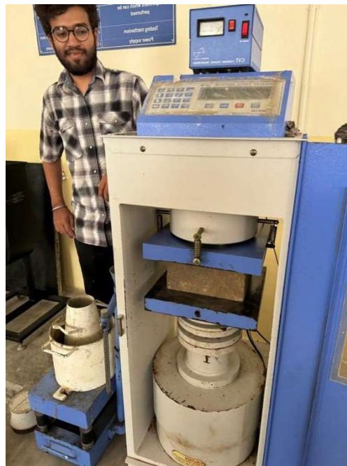
Fig 3.3: Compression testing machine (CPM) (KSSEM Laboratory)
