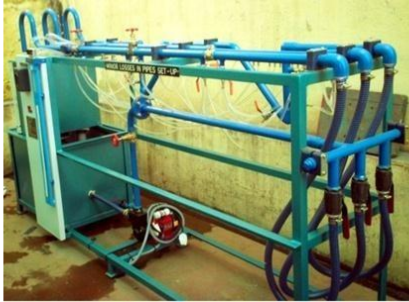
Fig: Frictional losses test rig
