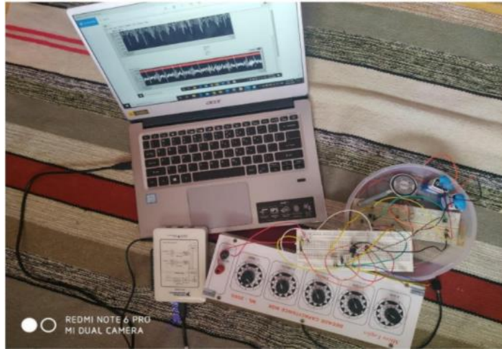
Figure: shows the Hardware implementation of the Filter along with the Acquisition and Pre-Amplification section
