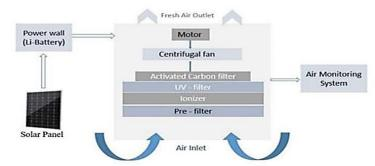
Fig 2.2 Solar powered air purifier with air quality monitoring system.
