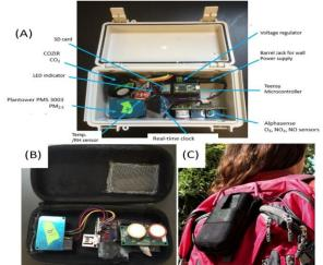
Fig 2.12. (a) All sensor package components in indoor/outdoor sampling case,(b) Personal monitoring case with internal components, and(c) Personal monitor hanging on a backpack.
