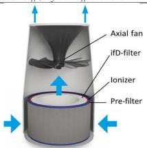
Fig 2.4 Easy handling air purifier
