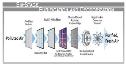
Fig 2.9 Design of Integrated Air purifier for Vehicle/homes
