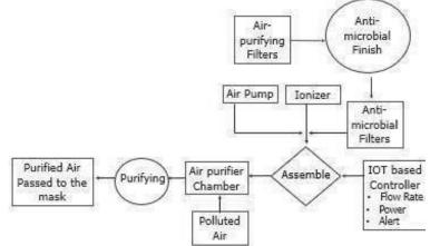
Fig 2.3 Flow chart for Advanced Air Purifier Facial mask
