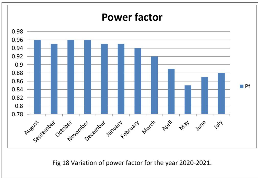
Figure 17 and 18 gives the variation of KVA and power factor for the year 2020 to 2021.
